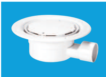
White Plastic Clamp Ring with Cover Plate and 1½" BS EN 1329-1:2000 solvent weld horizontal outlet. Overall height 75mm
