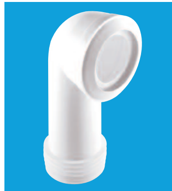
90° Bend (Long) 97-107mm Inlet 4"/110mm Outlet
