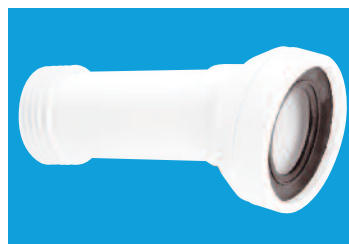
14° Angle Adjustable Length 97-107mm Inlet 3½"/90mm Outlet
