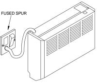
4. Isolate the electrical supply and connect the heater electric cable to the spur 3A). The fused spur must not be directly above the heater but should be accessible after the installation is complete.
