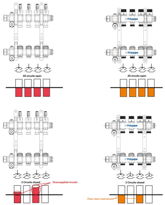
As circuits open and close the valve adjusts itself to ensure the set flow rate is maintained in each individual circuit, standard manifolds do not have this and as circuits open and close flow rates will move from the optimum set rate and oversupply some rooms.
