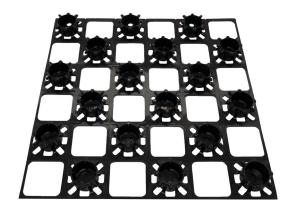
The panels interlock for easy storage and carrying and also form a precise grid for the pipe, ensuring that the minimum pipe bend radius is achieved. The unique design of the castellation incorporates fixing points in the centre which enables the panels to be mechanically fixed to the sub-floor and also acts to protect the pipe from damage caused by onsite foot traffic.
